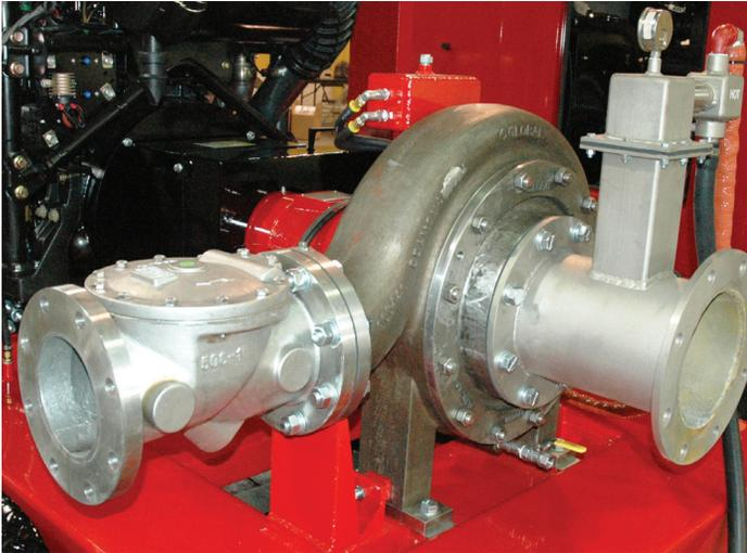
Pump wet end components made in CD4MCu offer superior corrosion resistance, hardness, and impact properties that make the alloy highly abrasion resistant in applications where pumps are subject to abrasive wear and chemical corrosion. Global Pump offers CD4MCu as an option for its entire Auto Prime line of efficient, rugged, heavy duty pumps. Popular models in stock. Contact us for more information. Varying DBA levels are available to meet design requirements.
