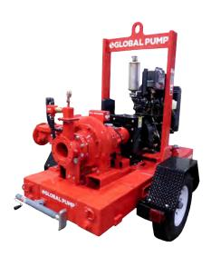
Global Pump® Standard Trash pumps are specifically designed to effectively handle a wide range of liquids from water to sewage and sludge that can contain solids and other material.
